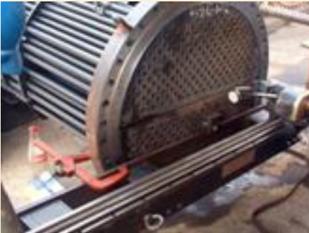
Exchanger Partition Milling
